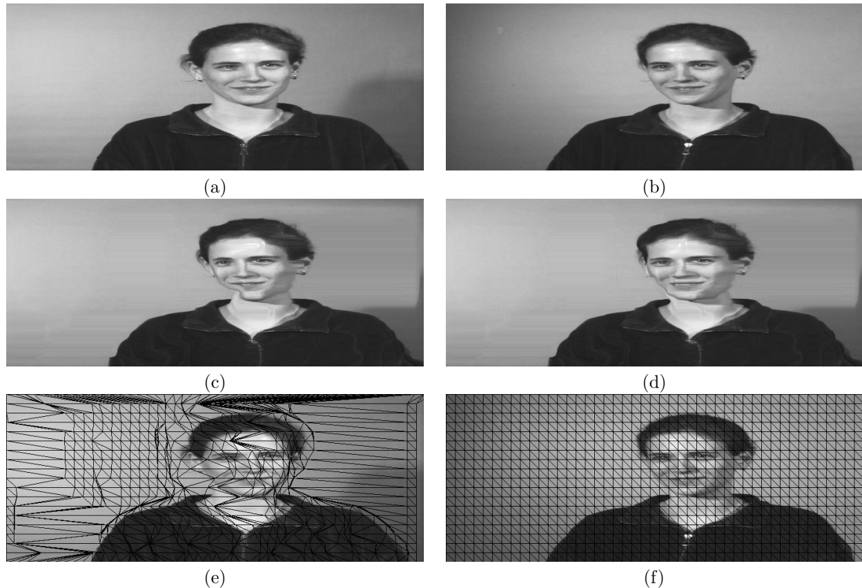
Figure 6. (a) Origin left frame of Anne #001. (b) Origin right frame of Anne #001. (c) Warped frame after the first stage. (d) Warped frame after the second stage. (e) The corresponding mesh of the left frame. (f) The regular mesh of the right frame.
